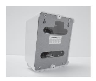
Our wall mount speaker is constructed using high quality ABS plastic (OFF-WHITE) with a slop of 15° suitable for used in hall, canteen, staircase, corridor, etc. Available with various tapping 100V line transformer (1W; 3W; 6W)
