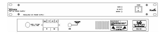
A 1 hu rack mounted unit, **PS-5424** provides constant and regulated 24V DC to the equipment requiring power source other than the ac mains.
