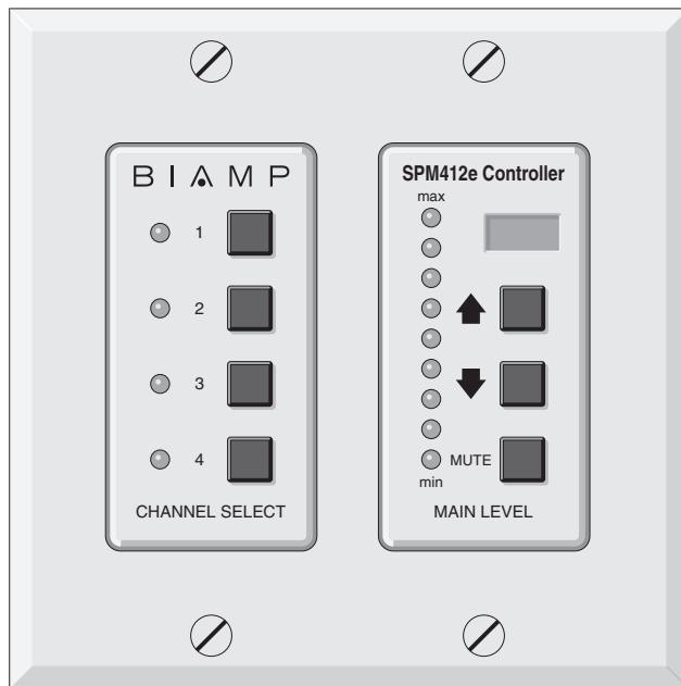
**The SPM412e Controller is an optional 'hard-wired' wall-mount control panel for the SPM412e Stereo Preamp/Mixer. The Controller includes a double-wide 'decorator' style electrical box, and provides control and indication of Channel Select and Main Level. The Controller is powered by the SPM412e and may be wired up to 2000 feet away, using 2-conductor shielded cable. The SPM412e Controller is covered by Biamp's five-year warranty.**
