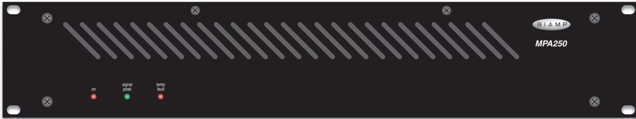
**MPA250 single-channel, multi-purpose amplifiers deliver a full 250 Watts of power into direct or distributed speaker systems. The MPA250 is designed for reliable service in permanent installations, and comes complete with short-circuit and thermal protection, including front/rear panel indicators and automatic reset. Plug-in barrier strip input and screw terminal outputs provide trouble-free, dependable connections. MPA250 amplifiers are UL listed and carry Biamp's five-year warranty.**
