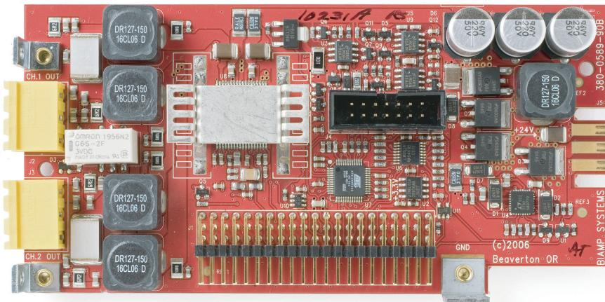
**PA-2 amplifier cards allow AudiaFLEX to directly power 4, 6, or 8 ohm speakers. The output power is software configurable from 5 to 30 watts dual-channel and from 10 to 60 watts mono-bridge. An upgraded AudiaFLEX power supply provides a total of 120 watts of power, for up to twelve PA-2 cards.**
