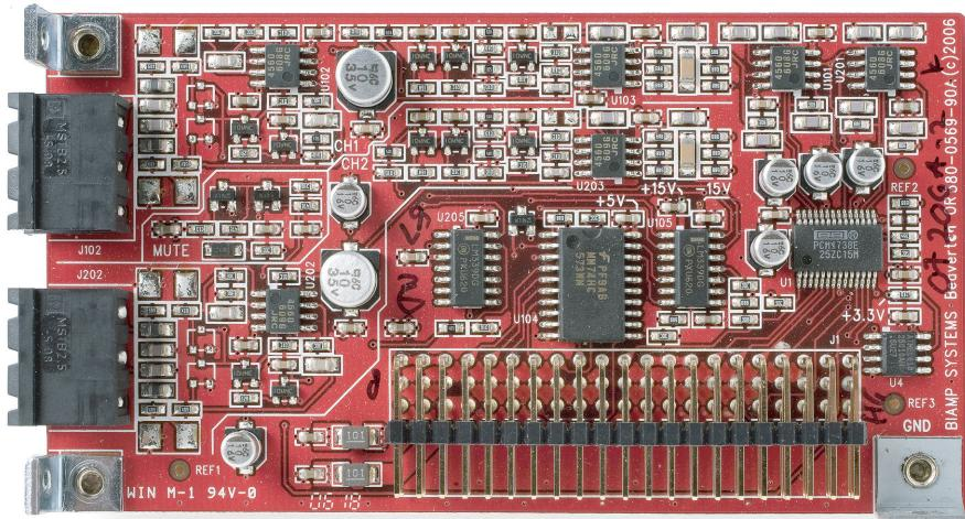
**OP-2e output cards allow each AudiaFLEX installation to have the quantity and type of outputs required. Each OP-2e Card provides two channels of mic/line output, as part of AudiaFLEX hardware. Outputs are balanced, and are provided on plug-in barrier strip connectors. Software control of individual outputs includes: mute; level; signal invert; and full-scale output reference.**
